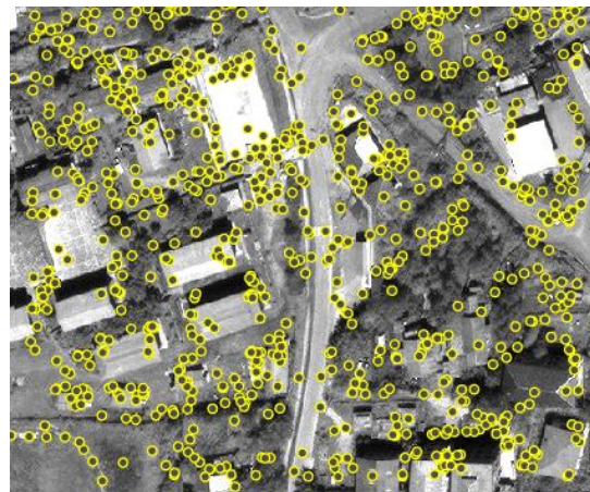
Figure 6: Final tie points generated for the specific region of the tested image.
